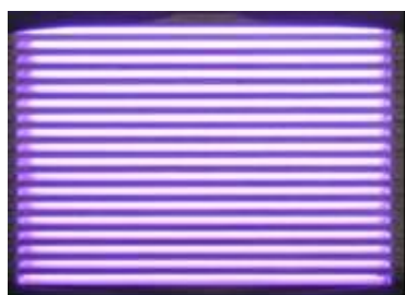
Figure 2: Photography of the plasma discharges in air.
