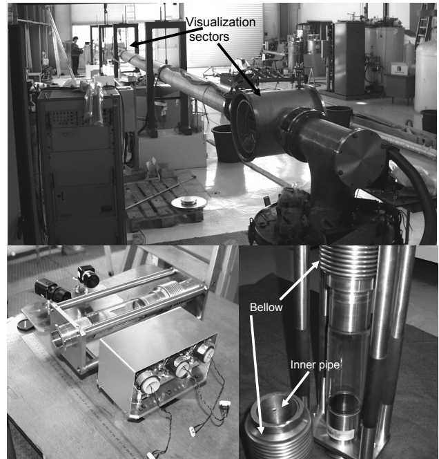
Fig. 3. The 22 m long He II cryostat and its two visualization sectors and below the lighting and CCD recording system located in the vacuum chamber to record flow motion. This tube is equipped with a thermal expansion compensation system using a bellow surrounding the two parts of a main tube to minimize flow perturbation.
