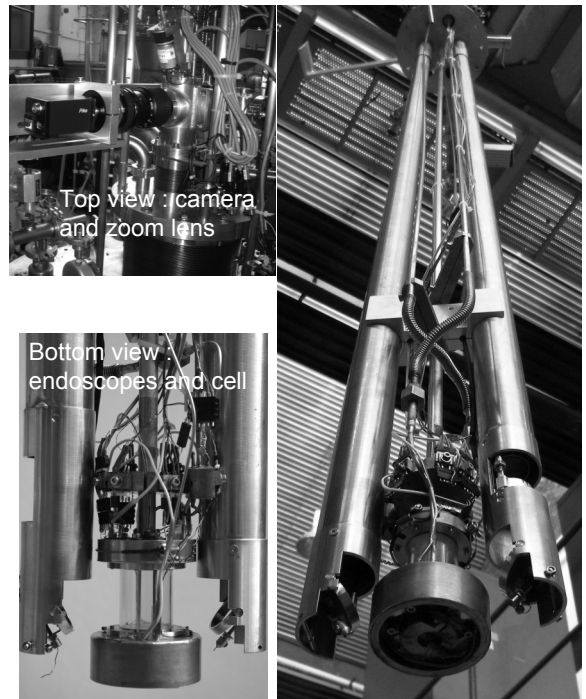
Fig. 8. Sketch of the optical system (and corresponding photos) in the anticryostat of OLGA experiment
