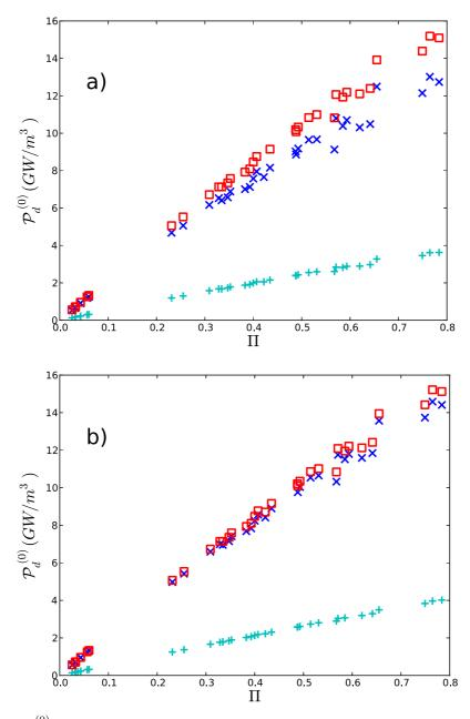
Figure 12:  $\mathcal{P}_d^{(0)}$  vs porosity associated with a semitransparent phase made of: i) Both steam and droplets of radius  $R_d = 50 \mu m$  (×) or  $R_d = 300 \mu m$  (+); ii) Only droplets of radius  $R_d = 50 \mu m$  ( $\Box$ );  $T_w = 2000 K$ ,  $T_v = 600 K$ ,  $f_v = 10^{-3}$  and  $p_v = 5 atm$  (a) or  $p_v = 1 atm$  (b).
