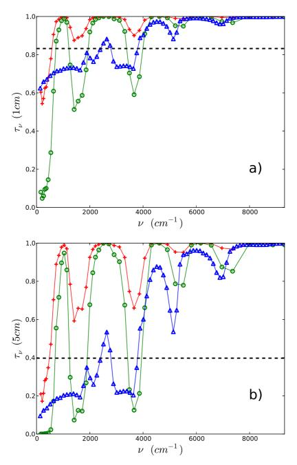
Figure 7: Transmissivity of columns of lengths 1cm (a) and 5cm (b) associated with interfaces (dashed line), water droplets at  $(R_d = 25 \,\mu m, f_v = 10^{-3})$  ( $\Delta$ ), steam at temperature  $T_v = 1000 \, K$  and pressure  $p_v = 1 \, atm$  ( $\times$ ) or  $p_v = 5 \, atm$  ( $\circ$ ).
