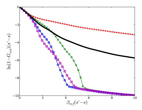
Figure 4: Extinction cumulative distribution function  $G_{ext}(s' - s, \theta = \pi/2, \varphi)$  for  $\theta = \pi/2$  and different  $\varphi$  values  $(1.5^{\circ} +, 16.5^{\circ} \times, 31.5^{\circ} \circ, 43.5^{\circ} \Box)$  and corresponding extinction cumulative function over all  $\varphi$  (thick line) [zone 2].
