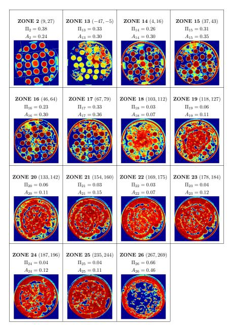
Figure 3:  $\gamma$ -tomographies of the zone 2 of PHEBUS-FPT1 and 14 zones of PHEBUS-FPT2, delimited axially by  $(z_{min}, z_{max})$  [mm] and associated values of  $\Pi$  and A [mm<sup>-1</sup>].
