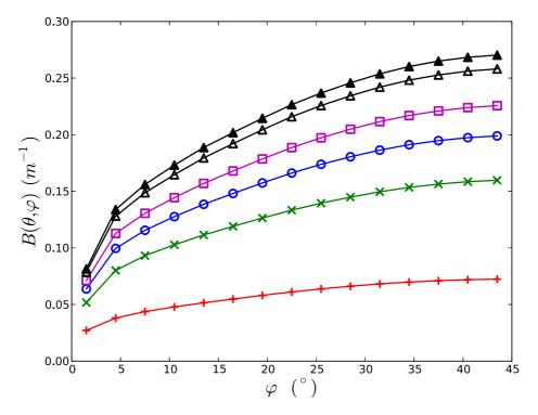
Figure 5: Directional generalized extinction coefficient at equilibrium  $[mm^{-1}]$  vs  $\varphi$  for different values of  $\theta$  (14.0° +, 34.1° ×, 44.9° °, 53.9°  $\Box$ , 69.3°  $\triangle$ , 90°  $\blacktriangle$ ) [zone 2].
