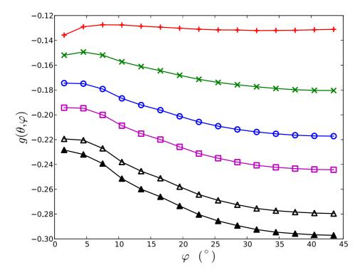
Figure 6: Directional scattering asymmetry parameter vs  $\varphi$  for different values of  $\theta$  (14.0° +, 34.1° ×, 44.9° °, 53.9°  $\Box$ , 69.3°  $\triangle$ , 90°  $\blacktriangle$ ) [zone 2].
