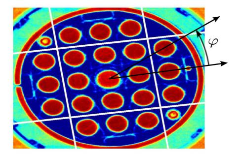
Figure 2: Example of image associated with a 2D cross-sectional  $\gamma$ -tomography; intact system (PHEBUS-FPT1, [26]).
