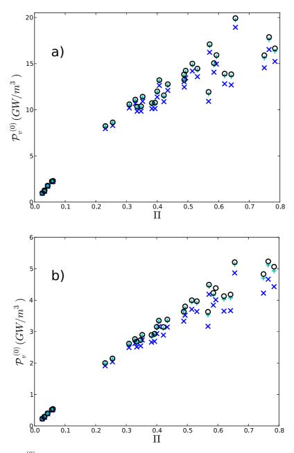
Figure 11:  $\mathcal{P}_{v}^{(0)}$  vs porosity associated with a semitransparent phase made of: i) Both steam and droplets of radius  $R_{d} = 50 \mu m$  (×) or  $R_{d} = 300 \mu m$  (+); ii) Only steam ( $\circ$ );  $T_{w} = 2000 K$ ,  $T_{v} = 600 K$ ,  $f_{v} = 10^{-3}$  and  $p_{v} = 5 atm$  (a) or  $p_{v} = 1 atm$ (b).
