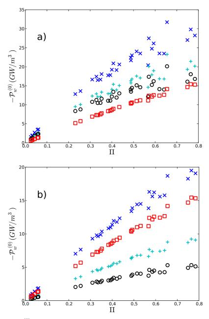
Figure 10:  $-\mathcal{P}_w^{(0)}$  vs porosity associated with a semitransparent phase made of: i) Both steam and droplets of radius  $R_d = 50\mu m$  (×) or  $R_d = 300\mu m$  (+); ii) Only steam ( $\circ$ ); ii) Only droplets of radius  $R_d = 50\mu m$  ( $\Box$ );  $T_w = 2000 K$ ,  $T_v = 600 K$ ,  $f_v = 10^{-3}$  and  $p_v = 5 atm$  (a) or  $p_v = 1 atm$  (b).
