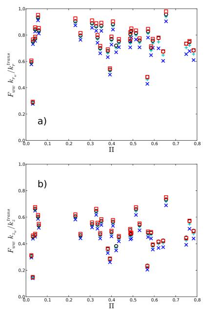
Figure 13: Dimensionless quantities  $F_{ww} k_{rw}/k_r^{trans}$  (a) and  $F_{ww} k_{zw}/k_z^{trans}$  (b) vs porosity associated with a semitransparent phase made of: i)Both steam and droplets of radius  $R_d = 50 \mu m$  (×) or  $R_d = 300 \mu m$  (+); ii) Only steam ( $\circ$ ); iii) Only droplets of radius  $R_d = 50 \mu m$  ( $\Box$ );  $T_w = 2000 K$ ,  $T_v = 600 K$ ,  $f_v = 10^{-3}$ ,  $p_v = 5 atm$ .
