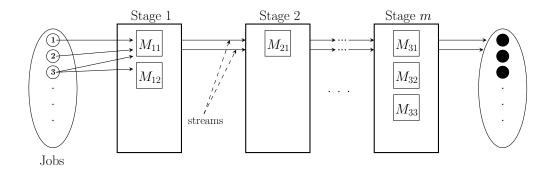
Figure 1: A hybrid flow-shop with multiprocessor tasks
