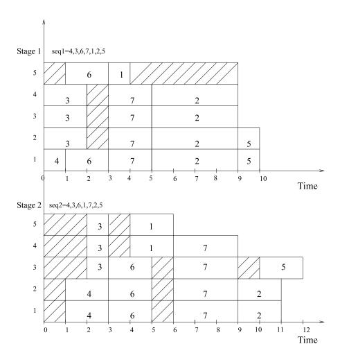
Figure 5: Gantt chart of the solution corresponding to Example 1 (solution decoded at first stage using a list scheduling algorithm; at second stage using a parallel schedule generation scheme)
