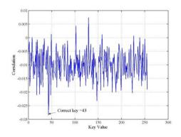
Figure 5. Illustration of secsseful SO-DPA attack secured by the CPNG with a number of traces 20480, the correct key *K*=43
