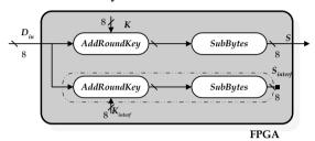
Figure 4. Implemnation of the beginning of the first AES iteration secured with CPNG countermeasure
