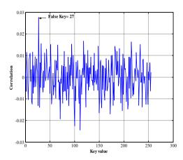
Figure 9. Illustration of unsecsseful SO-DPA attack on secured design by MCPNG countermeausre ,with a number of traces 20480, the correct key K=43
