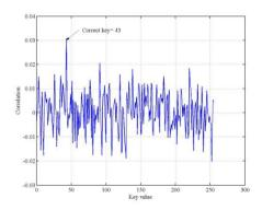
Figure 7. Successfull second order DPA attack on masking countermeasure with K= 43 and 20480 traces
