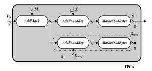
Figure 8. Implemnation of the beginning of the first AES iteration secured with MCPNG countermeasure
