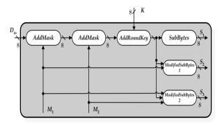
Figure 2. Hardware implmentation of multiple masking countermeasure
