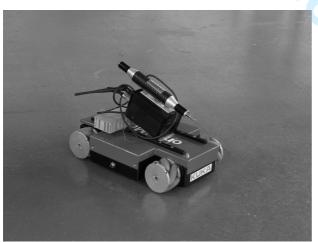
Figure 14 - Mini omniMove carrying an iGPS vector bar
