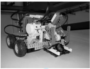
Figure 4 – Mobile robot carrying a laser tracker SMR
