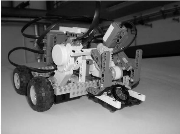
Figure 4 – Mobile robot carrying a laser tracker SMR
