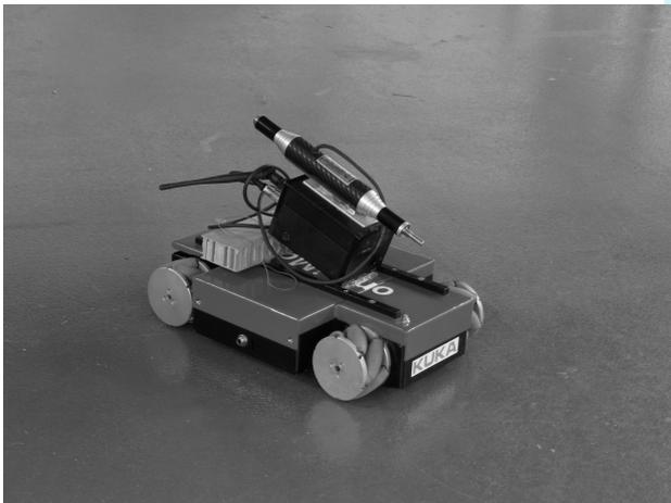
Figure 14 - Mini omniMove carrying an iGPS vector bar
