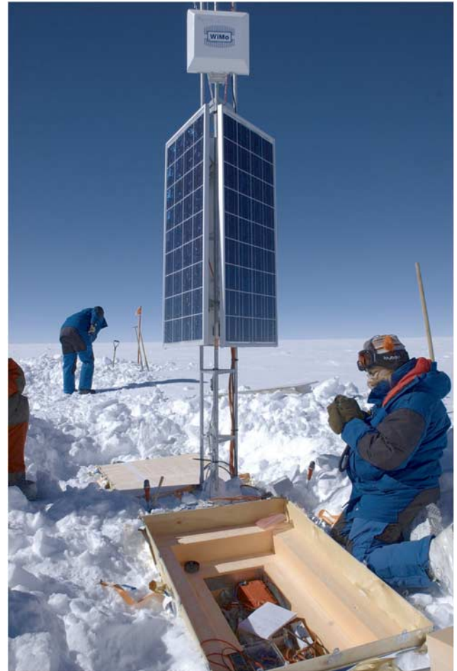
Fig. 2. Set-up of the autonomous seismological broadband station CAS03 inside the Antarctic continent, 5 km away from Dome C.
