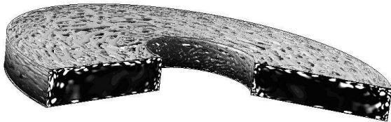
Figure 4: Iso-surfaces of the Q-criterion and iso-lines in the meridian planes. LES-FD.
