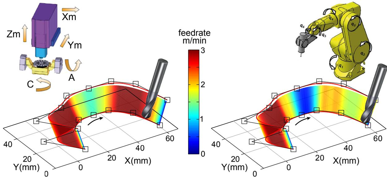
Figure 9: Open pocket with 5-axis machine and robot arm.
