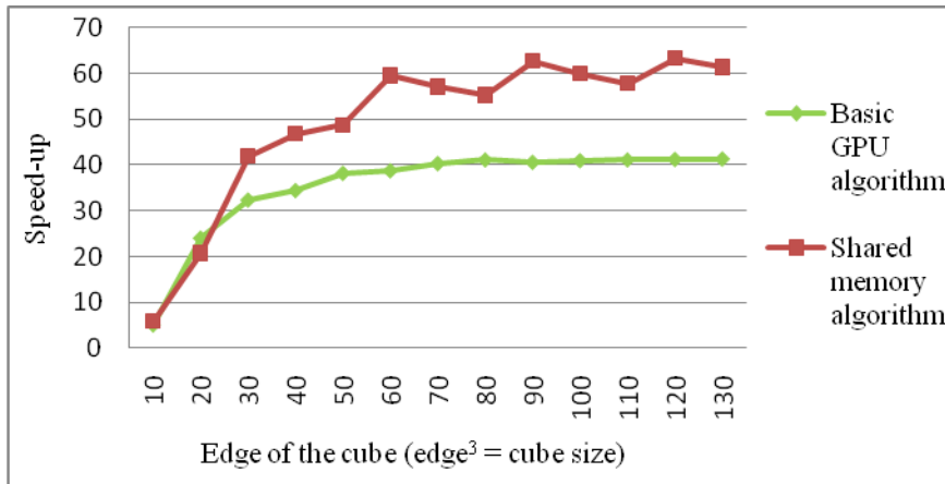
Figure 10: Comparison of speed-up evolution for 1000 iterations depending on the cube sizes (50 measures for each point).
