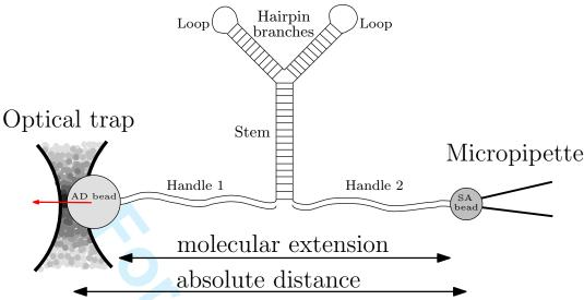
Figure 2. Sketch of the experimental setup. In our experiments we measure the relative distance X rather than its absolute
