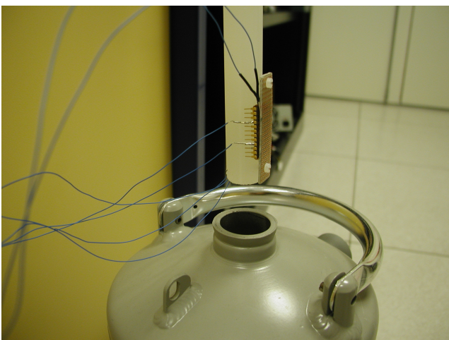
Fig. 5 Cold temperatures are obtained through the use of liquid nitrogen and a rod
