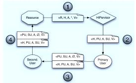
Figure 3: SPKI authorization certificate flow when a secondary user joins an existing VPXI.
