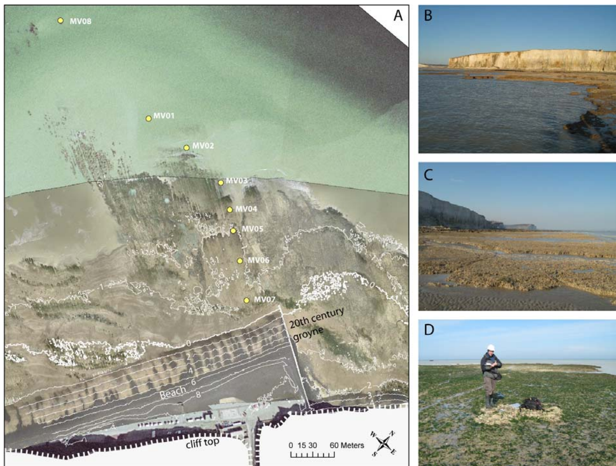
Figure 1. A. Aerial photograph of Mesnil Val site. Sample locations are shown; contour levels are drawn each meter (aerial LIDAR data), the 0 level (NGF reference) in bold (average water level is +0.43m NGF). Note the groyne dating back to the 20th century has had no long term effect on platform downwearing, but is clearly the cause of beach accumulation to the southwest. The photograph is not taken at very low tide, explaining the fact that all sampling sites are submerged. The cliff height is ~20 m, reaching 50-80 m less than 1 km away either northeast or southwest. B. to D. Site photos. Photo D. is the MV04 sampling site.
