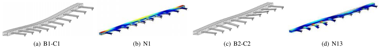
Figure 1.6: Eigenmode shapes of analytical mode and FEM mode
