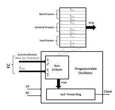
Fig. 9. Memory mapping of the programmable oscillator. It selects the PSTR programming code to apply in function of a given frequency level calculated by the digital controller.
