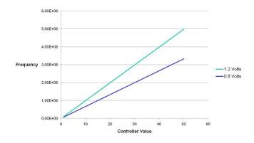
Fig. 7. Behavioral variation of the frequency controller with respect to the input voltage values.
