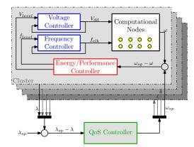
Fig. 4. Automatic control are essential in nanometric chips to manage the computational activity and energy consumption. Three overlapped loops are hence introduced: the voltage and frequency control (low-level), the energy-performance tradeoff control (middle-level) and the applicative quality of service control (high-level).
