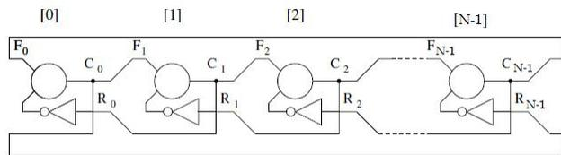
Fig. 8. Representation of a possible CMOS implementation of a self-timed ring, whose each stage is composed of a C-element and an inverter.
