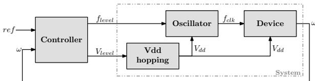
Fig. 10. Representation of the system architecture to control the energy-performance tradeoff. The controller calculates the control variables (voltage level  $V_{level}$  and frequency level  $f_{level}$ ) from the error between the measured computational speed  $\omega$  and a given setpoint  $ref$ , and sends them to both actuators (the Vdd-hopping and the ring oscillator respectively).
