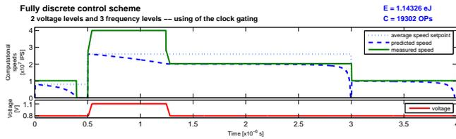
(a) Simulation results with three frequency levels, one for the high voltage level and two for the low one, and the clock-gating principle.
