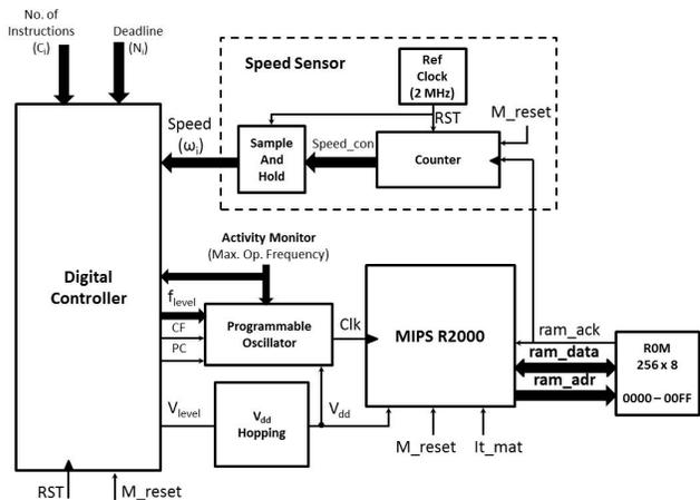
Fig. 6. Architecture of the controlled system in the MIPS environment. The digital controller calculates the voltage and frequency levels to send to the V<sub>dd</sub>-hopping and the programmable oscillator in order to manage the energy-performance tradeoff of the MIPS R2000. A speed sensor is also used to provide the real-time computational speed.
