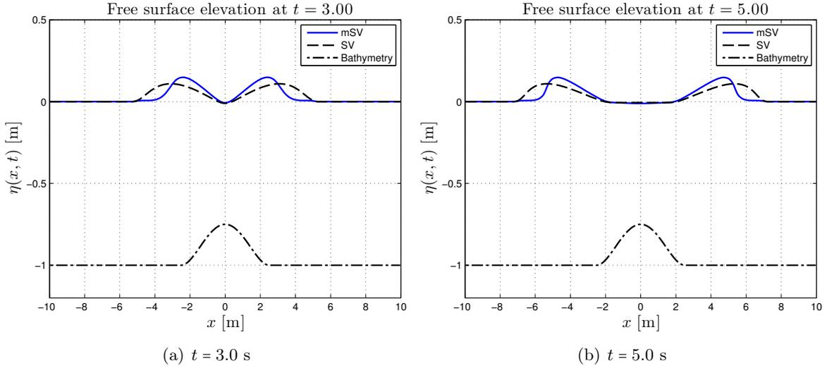
**Figure 16.** *Fast bottom uplift test-case ( $\alpha_2 = 12$ ).*
