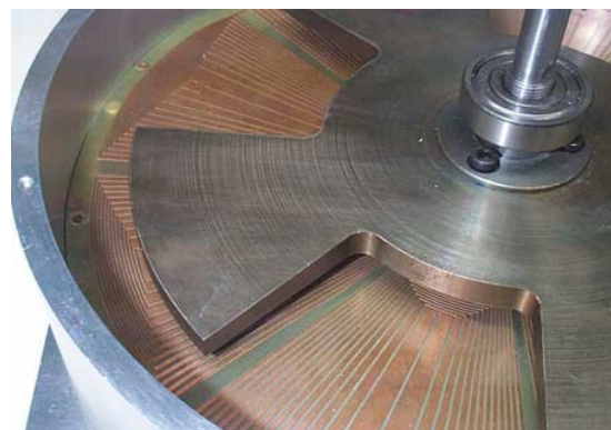
Fig. 3: Upper side of the machine (only the armature winding is visible)
