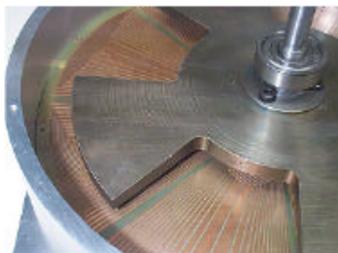
Fig. 23: ( \Phi = 20 cm) Upper side of the machine (only the armature winding is visible)
