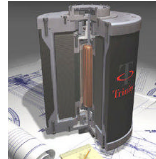
Fig. 17: The AFS-Trinity system 200 kW - 2 kWh mass: 540 kg 40,000 rpm 100,000 cycles
