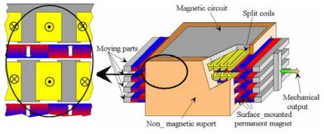
Fig. 3: Split-coil multi-airgap architecture (3) and 3D view of one phase of an actuator
