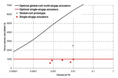
Fig. 24: Comparison of scale effect between optimisation results and actual actuators
