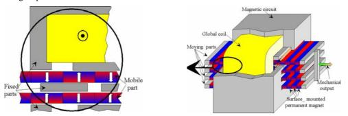
Fig. 4a: Global-coil multi-airgap architecture (4) and 3D view of one phase of an actuator with mobile permanent magnets
