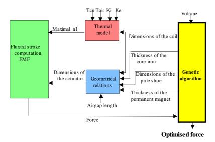
Fig. 14: Global diagram of the optimisation algorithm
