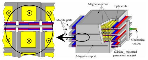
Fig. 2: Multi-motor architecture (2) and 3D view of one phase of an actuator
