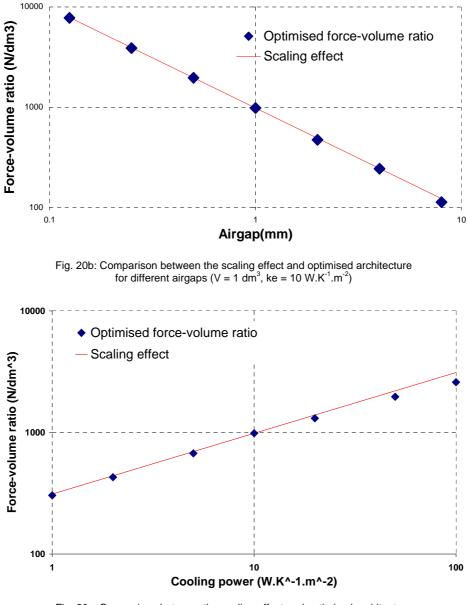
Fig. 20c: Comparison between the scaling effect and optimised architecture for different cooling powers (V = 1  $dm^3$ , g = 1 mm)
