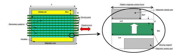
Fig. 13: Global dimensions and pattern dimensions
