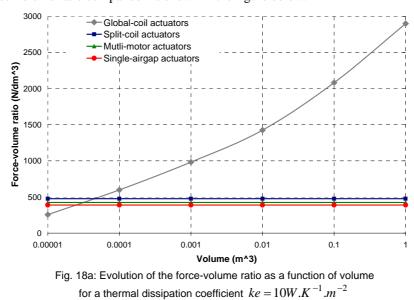
The force-volume ratio comparison is shown in the figure below:
