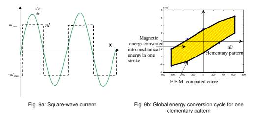
The area  $W_m$  of the cycle represents the transfer from electrical energy to mechanical energy at each step  $\tau$  of the actuator. In the case of the ideal square-current supply, we obtain:
