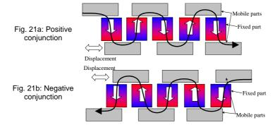
Fig. 21: Elementary cell of the multi-airgap actuator
