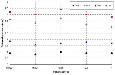
Fig. 16a: Optimised dimensions for the global-coil multi-airgap actuator as a function of global volume
