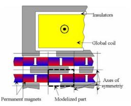
Fig. 7: Axes of symmetry for the global-coil multi-airgap actuator
