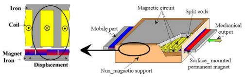
Fig. 1: Basic single-airgap architecture (1) and 3D view of one phase of an actuator
