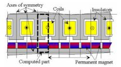
Fig. 6: A portion of the multi-motor architecture with the 2D Finite Element-modelled part (see Figure 2)
