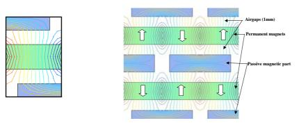
Fig. 16b: Optimised elementary pattern of a global-coil multi-airgap actuator and detail of the optimised actuator in conjunction
