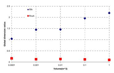
Fig. 16c: Global dimension ratio for the global-coil multi-airgap actuator as a function of global volume
