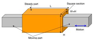
Fig. 11: Shape of square-section actuators
