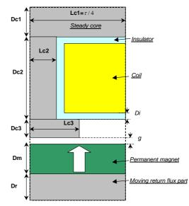
Fig. 12: The geometrical parameters of a pattern
