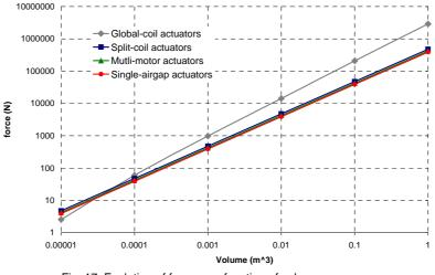
Fig. 17: Evolution of force as a function of volume
