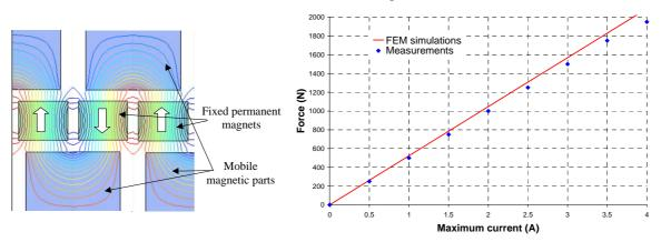
Fig. 23a: Finite Element Method simulation of an elementary pattern
