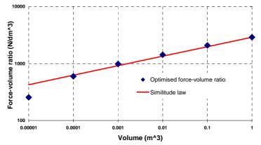
Fig. 20a: Comparison between the scaling effect and optimised architecture For for different volumes (g = 1 mm,  $\lambda_{th}$  = 10 W.K<sup>-1</sup>.m<sup>-2</sup>)
