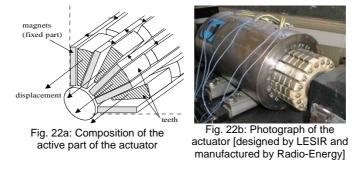
Fig. 22: Example of a permanent magnet reluctance multi-airgap actuator
