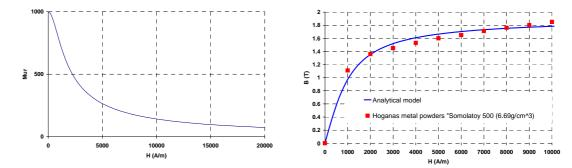
Fig. 8: Relative permeability curve and saturated B(H) curve for Hoganas® SOMALOY 500 soft magnetic composites (parameters of the model are :  $B_{sat} = 1.6T$  and  $\mu_{r_{max}} = 1000$ )
