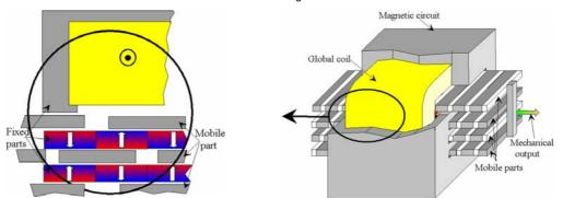
Fig. 4b: Global-coil multi-airgap architecture (4) and 3D view of one phase of a fixed permanent magnet actuator
