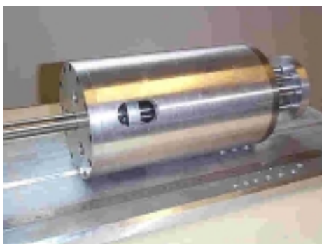
Fig. 1: The multi-airgap linear actuator prototype
