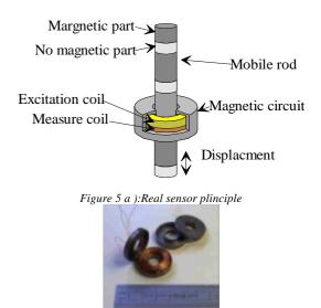
Fig 5 b) :magnetic ring prototypes
