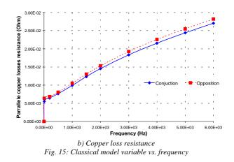
Both magnetization inductance and copper loss resistance depend on the frequency and the position.
