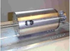
Fig. 1:The multi-airgap linear actuator prototype
