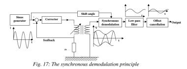
For synchronous demodulation, the choice of shift angle must yield maximal sensor sensitivity, which means maximal output magnitude between two extreme positions (a half-step displacement of the rod) (see Figure 18).
