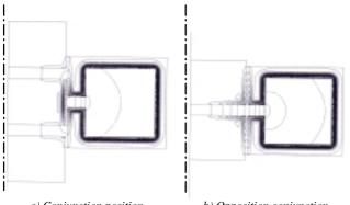
a) Conjunction position b) Opposition conjunction Fig. 9: High-frequency (1.5 kHz) field map  $\mu_r = 120, \rho = 1.4.10^{-7} \Omega.m$
