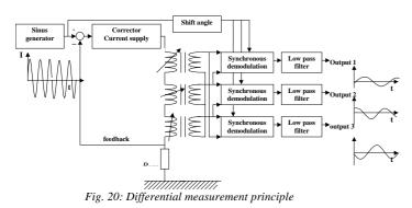
It immediately cancels the offset output signal value, without any adjustment. Moreover, it protects against temperature sensitivity.
