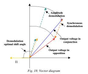
Synchronous demodulation combines the amplitude variation and the angle variation between the two extreme positions.
