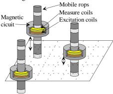
Fig. 6: Relative positions of the three sensors
