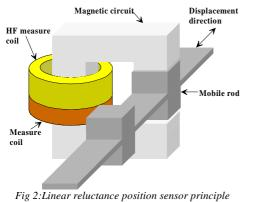
Fig 2. Linear relaciance position sensor principle
