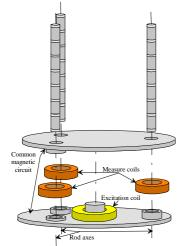
Fig. 22: Close-up view of the common excitation coil structure
