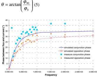
Fig. 13: Phase between the current and the flux
