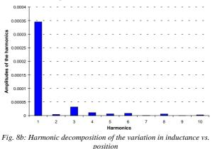
It can be observed that the variation in inductance displays few harmonics. According to our initial approach, we consider this variation as a pure sinus variation; hence, the relation between position and output signals will be simpler.
