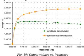
Hence, synchronous demodulation always yields better results, yet with the disadvantage of a more complex demodulation circuit; we have chosen this last type.
