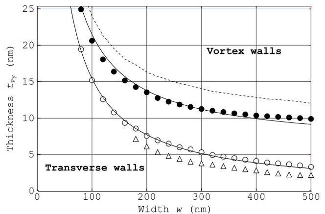
FIG. 2. Phase diagram of head-to-head domain walls in stripes, with the boundary between symmetric and asymmetric TWs ( $\Delta$ ) and TW and VW ( $\circ$ ) in a single layer, and asymmetric TW and VW in a spin valve ( $\bullet$ ). From bottom to top, the three lines are: a  $1/t_{Py}$  fit to the TW-VW data for a single layer, a thickness translation of the former to fit the TW-VW data for a spin valve, and another thickness translation with  $t_{sh}(t_{Cu} = 0)$ , see Eq. (3) and text.
