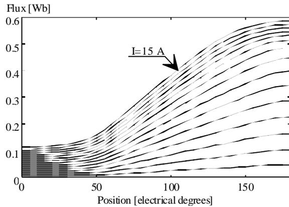
Fig. 3: Deduced flux linkage from the static torque
