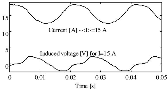
Fig. 10: Current and induced voltage shapes
