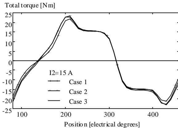
Fig. 5: Total torque for different feeding cases
