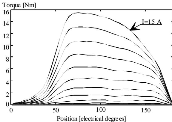
Fig. 2: Static single phase electromagnetic torque characteristics
