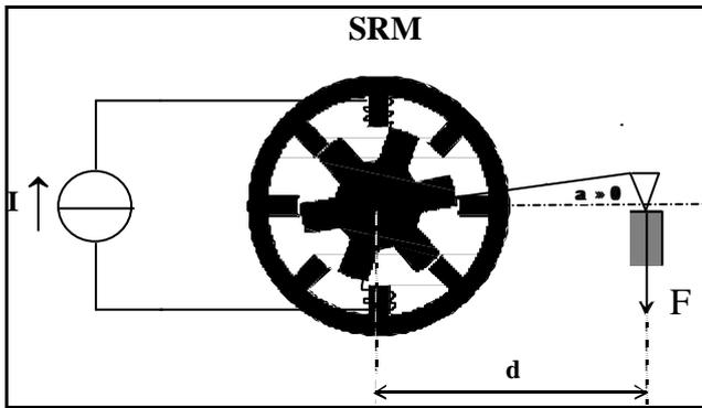
Fig. 1: Static torque measurement bench
