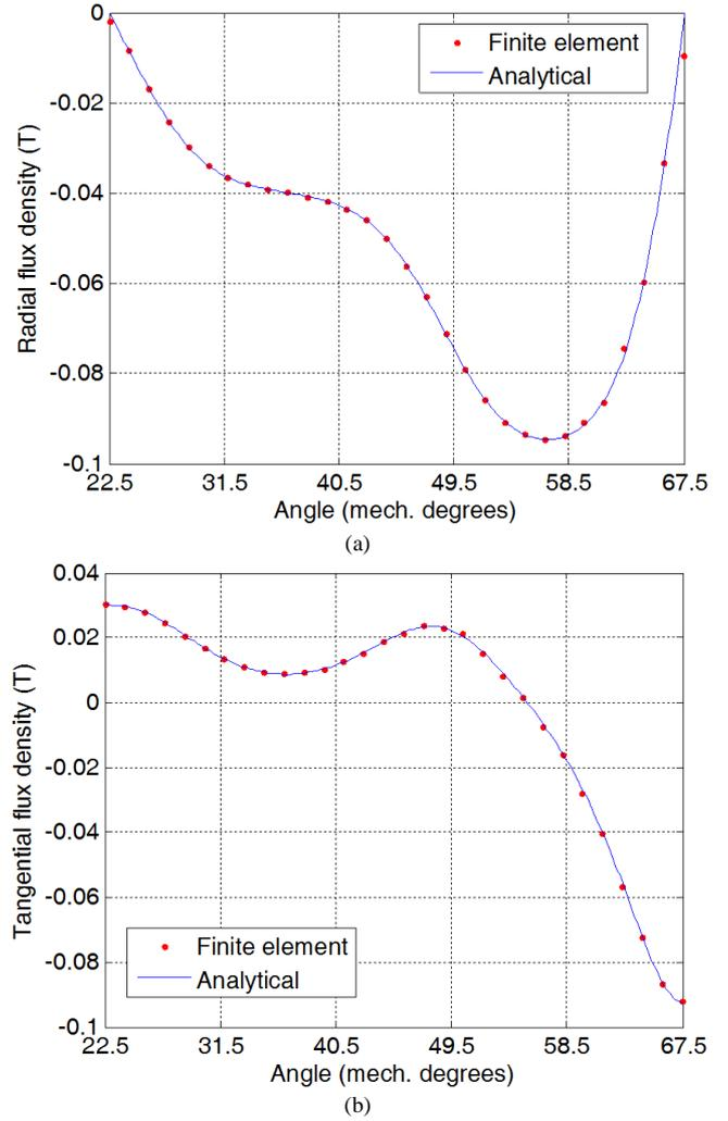
Fig. 12. Flux density distribution for radial (a) and tangential (b) components of armature reaction in the 1<sup>st</sup> PMs region ( $k=1$ ) at  $r = (R_1 + R_2)/2$ .
