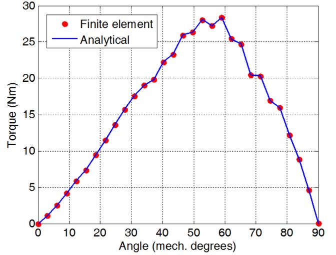
Fig. 18. Static torque versus rotor position for  $J_{rms}=4\text{A/mm}^2$ .
