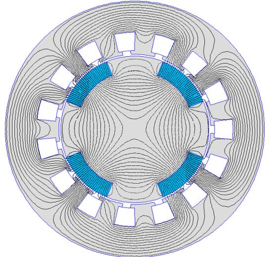
Fig. 5. Magnetic flux distribution for no-load condition obtained with FEM.
