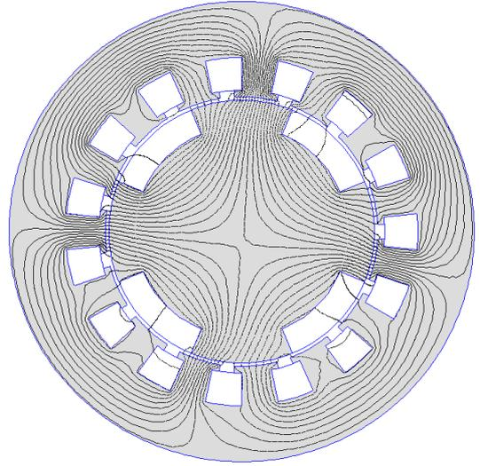
Fig. 10. Armature reaction magnetic flux distribution obtained with FEM for  $J_{rms} = 4A/mm^2$  (the magnets are removed).
