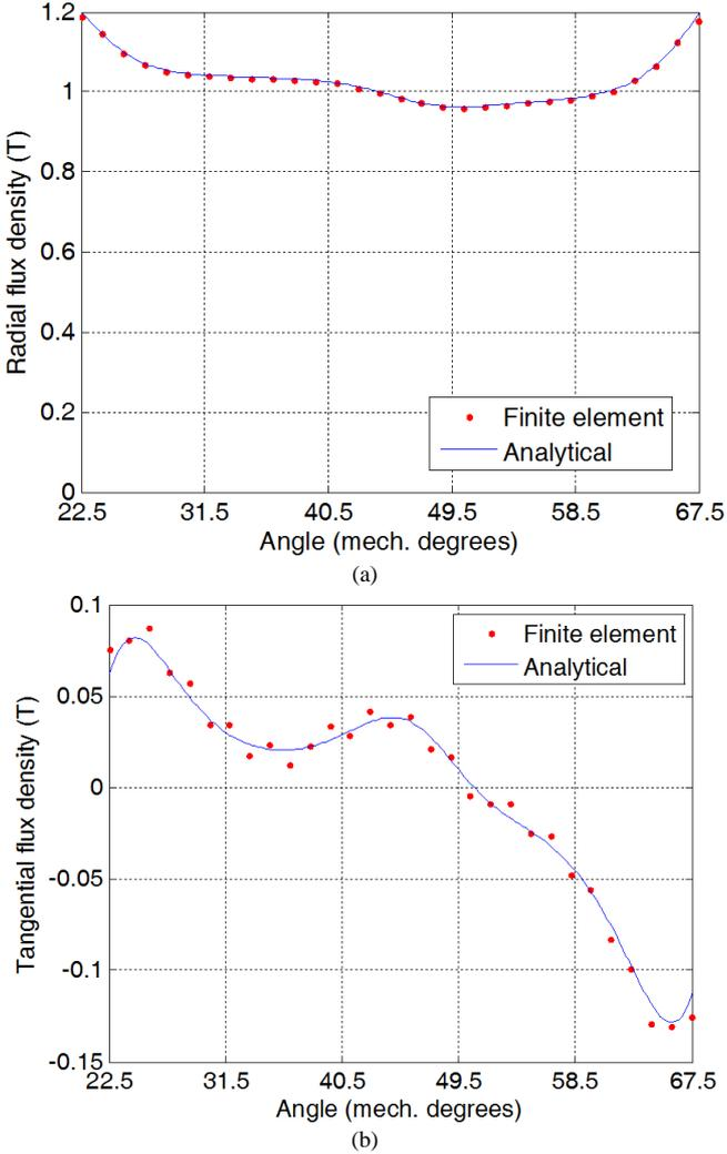
Fig. 17. Flux density distribution for radial (a) and tangential (b) component in the 1<sup>st</sup> PMs region ( $k=1$ ) at  $r=(R_1+R_2)/2$  for load condition.
