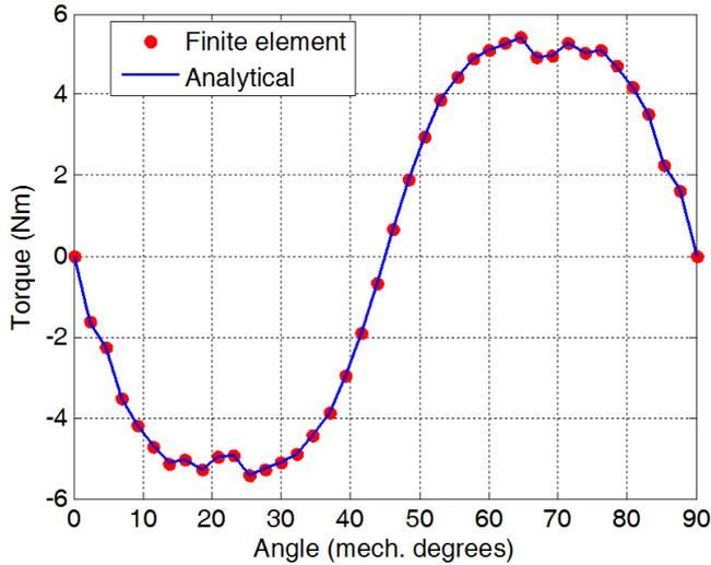
Fig. 13. Static torque versus rotor position due to slots currents alone (reluctance torque) for  $J_{rms}=4 A/mm^2$ .
