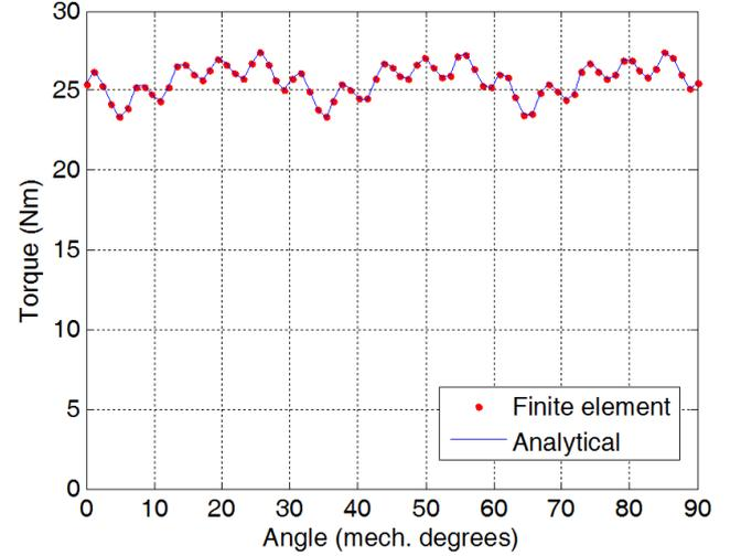
Fig. 19. Electromagnetic torque versus rotor position for  $J_{rms}=4\text{A/mm}^2$ .
