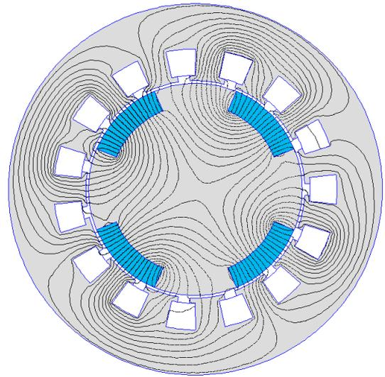
Fig. 15. Magnetic flux distribution for load condition.
