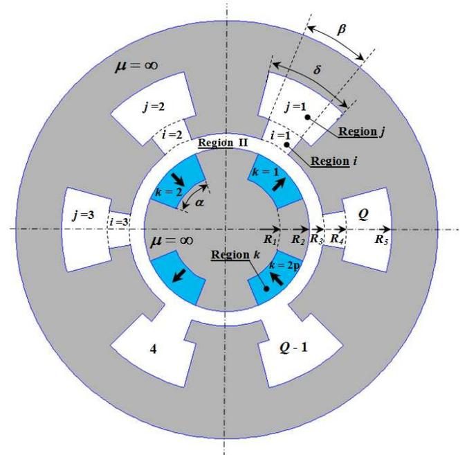
Fig. 1. Surface-inset permanent magnet motor with semi-closed slots ( $p = 2$  and  $Q = 6$ ).
