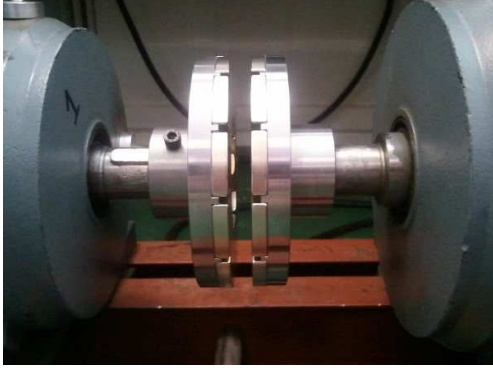
Fig. 13. Axial magnetic coupling prototype placed on the test bench ( e = 9.5\text{mm} ).
