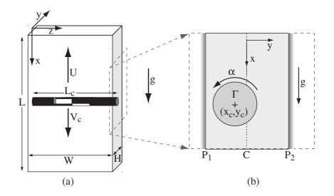
Figure 1. Experimental setup. a) Front view - U: mean flow velocity,  $V_{cx}$ : vertical component of the cylinder velocity. b) Side view -  $y_c$ : transverse position of the center of mass of the cylinder,  $\Gamma$ : Torque.
