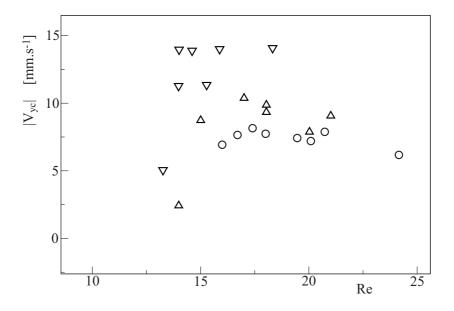
Figure 6. Maximum velocity  $|V_{cy}|^0$  of the transverse oscillations inside the gap as a function of the Reynolds number Re defined by Eq. 1. ( $\triangle$ ), ( $\circ$ ): PMMA cylinders of respective diameters D = 1.45 and D = 1.63 mm in solution N1. ( $\nabla$ ): carbon cylinder in solution N2 (D = 1.45 mm).
