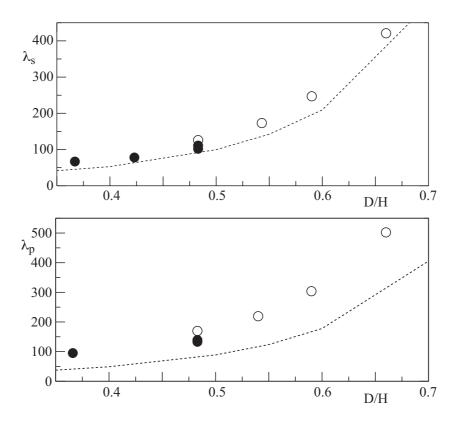
Figure 4. Top: Variations of  $\lambda_s$  (top) and  $\lambda_p$  (bottom) vs D/H. ( $\circ$ ),( $\bullet$ ) : experimental values of  $\lambda_s$  (top) and  $\lambda_p$  respectively with and without oscillations; dashed lines: numerical data from ref.<sup>9</sup> (for  $\lambda_s$ ) and ref.<sup>8</sup> (for  $\lambda_p$ ).
