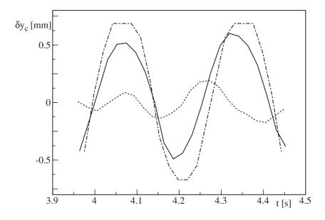
Figure 5. (a) variation of the transverse deviation  $\delta y_c$  of a PMMA cylinder (D = 1.45 mm) in the gap as function of time for different mean velocities U of solution N1. Dashed line: ( $U = -2 \text{ mm.s}^{-1}$ , Re = 14), solid line: ( $U = -4 \text{ mm.s}^{-1}$ , Re = 15), dashed dotted line: ( $U = -12 \text{ mm.s}^{-1}$ , Re = 19).
