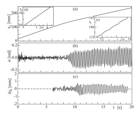
Figure 2. Experimental measurements obtained using solution N1 (see Tab. I) with D = 1.45 mm (D/H = 0.48) and U = -10.55 mm.s<sup>-1</sup>. (a)  $x_c$  vs time t (s). (b)  $\alpha$  vs t. (c)  $\delta y_c$  vs t.
