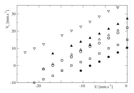
Figure 3. Vertical velocity  $V_{cx}$  of cylinders of diameter D in solutions N1 or N2 (see Tab. I) as a function of the fluid velocity U. Open symbols: oscillating cylinders; solid symbols: no oscillations. PMMA cylinders -  $(\triangle)$ ,  $(\blacktriangle)$ : D = 1.45 mm (D/H = 0.48), N1;  $(\circ)$ ,  $(\bullet)$ : D = 1.63 mm(D/H = 0.54), N1 for  $(\circ)$  and N2 for  $(\bullet)$ ;  $(\Box)$ : D = 2.1 mm (D/H = 0.7), N1. Carbon cylinder - $(\nabla)$ : D = 1.45 mm (D/H = 0.48), N2.
