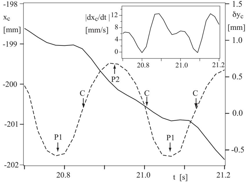
Figure 8. Time variation of the vertical coordinate  $x_c$  (solid line) and of the transverse displacement  $\delta y_c$  (dashed line) as a function of time for the same experiment as in Fig. 7. Inset : variation of the absolute value vertical velocity  $V_{cx} = dy_c/dt$  as a function of time.
