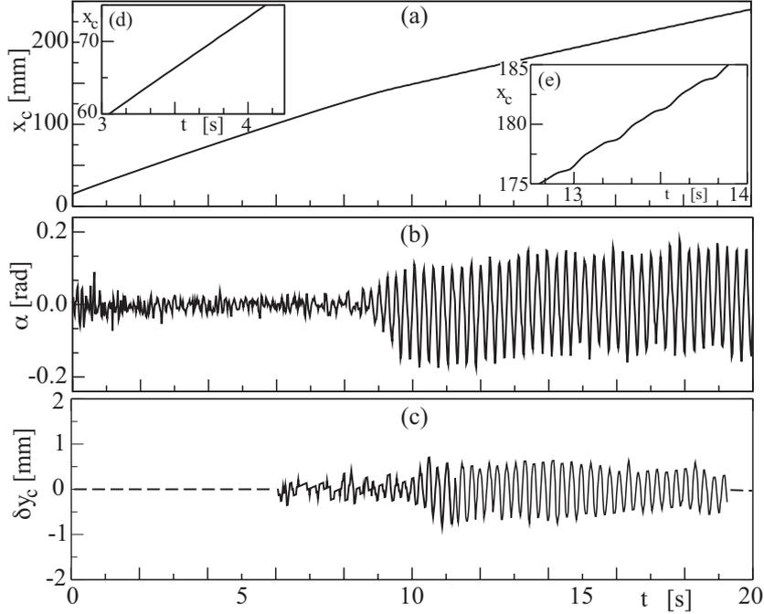
Figure 2. Experimental measurements obtained using solution *N1* (see Tab. I) with  $D = 1.45$  mm ( $D/H = 0.48$ ) and  $U = -10.55$  mm.s $^{-1}$ . (a)  $x_c$  vs time  $t$  (s). (b)  $\alpha$  vs  $t$ . (c)  $\delta y_c$  vs  $t$ .
