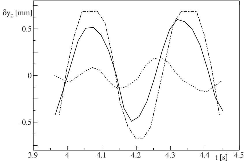
Figure 5. (a) variation of the transverse deviation  $\delta y_c$  of a PMMA cylinder ( $D = 1.45$  mm) in the gap as function of time for different mean velocities  $U$  of solution  $N1$ . Dashed line: ( $U = -2$  mm.s $^{-1}$ ,  $Re = 14$ ), solid line: ( $U = -4$  mm.s $^{-1}$ ,  $Re = 15$ ), dashed dotted line: ( $U = -12$  mm.s $^{-1}$ ,  $Re = 19$ ).
