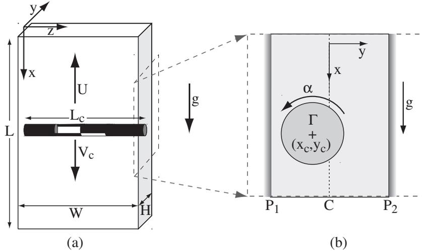
Figure 1. Experimental setup. a) Front view -  $U$ : mean flow velocity,  $V_{cx}$ : vertical component of the cylinder velocity. b) Side view -  $y_c$ : transverse position of the center of mass of the cylinder,  $\Gamma$ : Torque.
