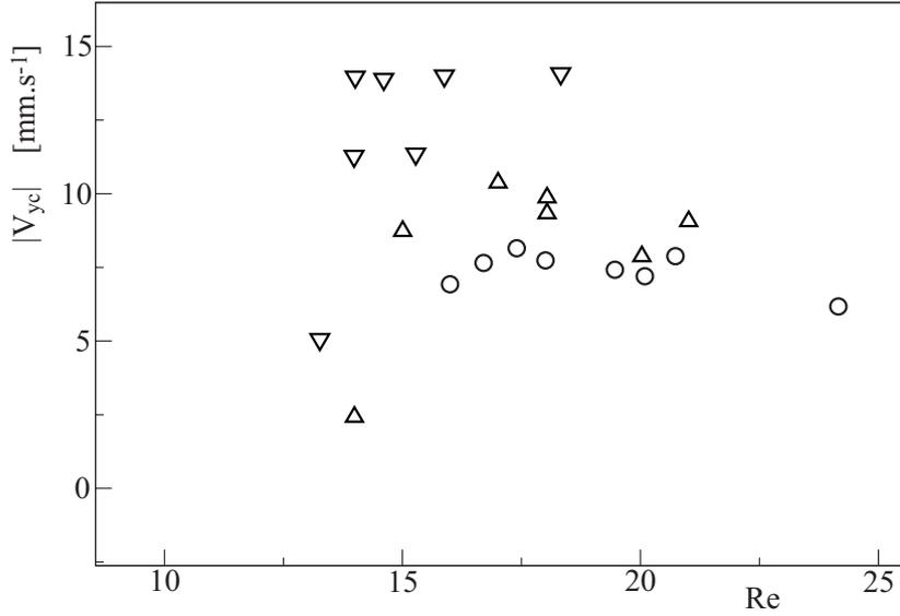
Figure 6. Maximum velocity  $|V_{cy}|^0$  of the transverse oscillations inside the gap as a function of the Reynolds number  $Re$  defined by Eq. 1. ( $\Delta$ ), ( $\circ$ ): PMMA cylinders of respective diameters  $D = 1.45$  and  $D = 1.63$  mm in solution  $N1$ . ( $\nabla$ ): carbon cylinder in solution  $N2$  ( $D = 1.45$  mm).
