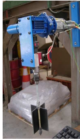
Figure 1. Schematic diagram of the experimental setup (left) – View of the high torque vane rheometer (right).
