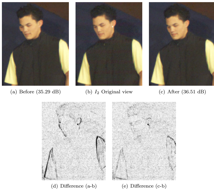
Fig. 9. Comparison of a synthesized virtual view without and with floating geometry.
