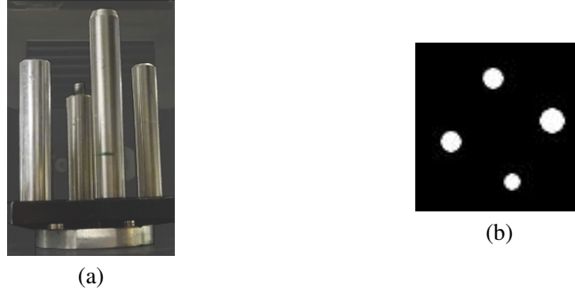
Fig. 7. (a) Object composed of four metallic bars (two bars diameter 10mm on the top and on the left, one bar diameter 12mm on the right and one bar diameter 8mm on the bottom), (b) Synthetic model of the object.
