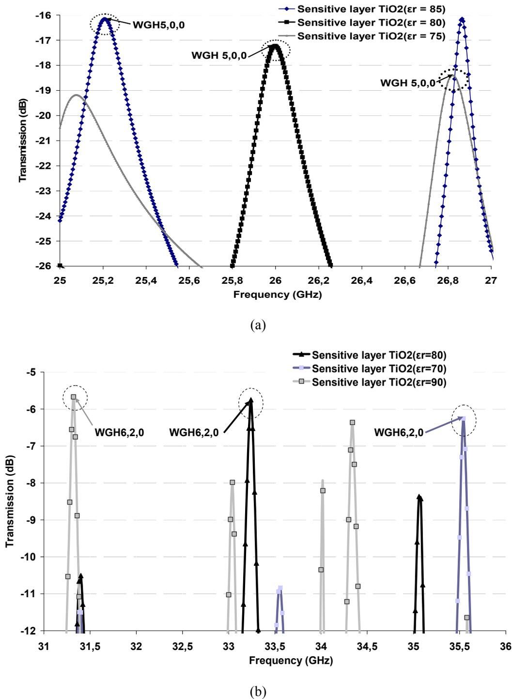
**Fig. 4.** Transmission coefficient from port 1 to port 3 versus frequency for various DR relative permittivities: (a) Permittivity  $\epsilon_r = 75, 80$  and  $85$ ; and (b) Permittivity  $\epsilon_r = 70, 80$  and  $90$ .
