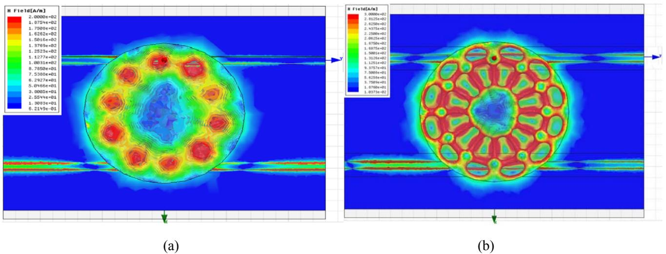
**Fig. 3.** Simulated magnitude of the magnetic field at the resonant frequency of the: (a) WGH<sub>5,0,0</sub> mode (at 26.01 GHz); and (b) WGH<sub>6,2,0</sub> mode (at 33.34 GHz)
