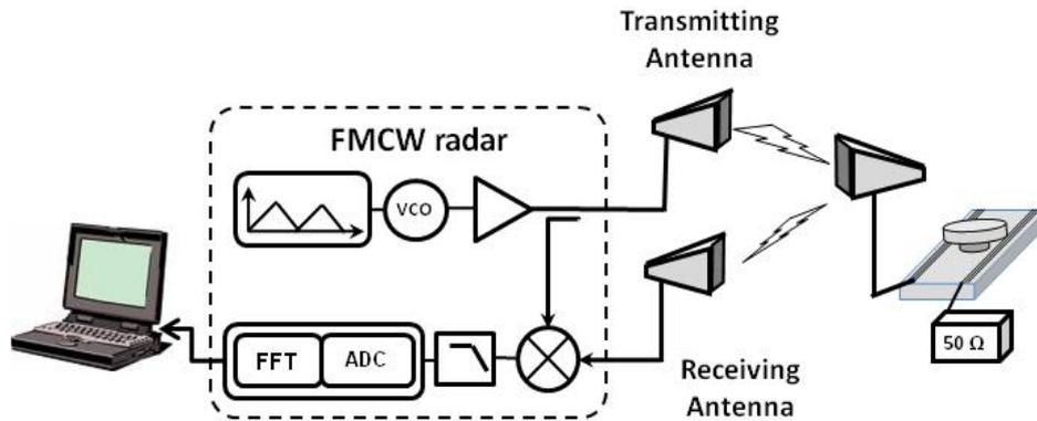
**Fig. 9.** Block diagram of the FMCW radar system.
