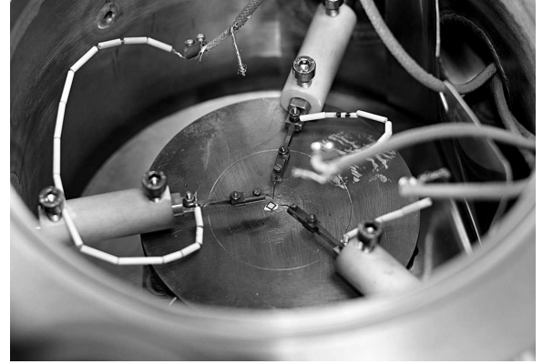
Fig. 6. Picture of the vacuum probe station (with top cover removed) showing the diode under test, directly bonded to the temperature-controlled chuck and the three probes (the fourth is directly connected to the chuck)
