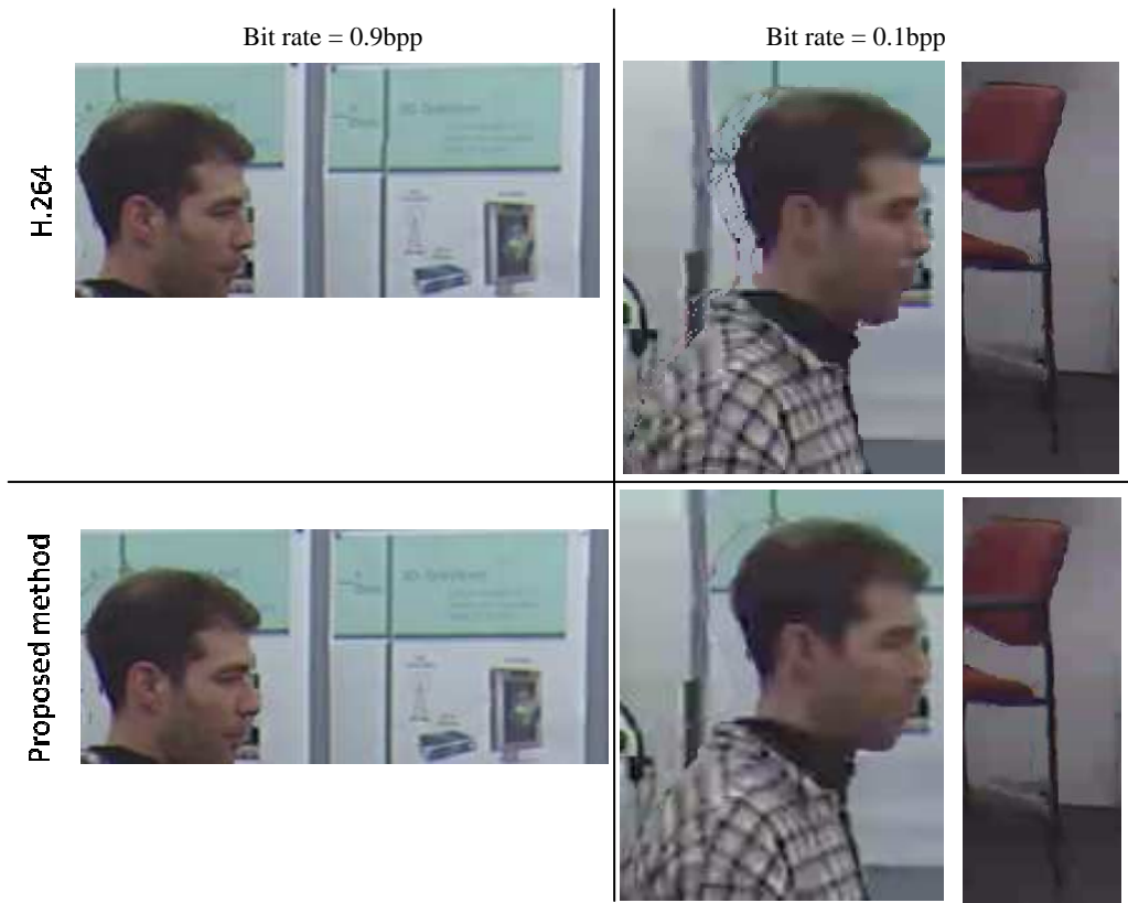
Figure 9: Snapshots of synthesized views from data encoded with H.264 and from data encoded with the proposed method.
