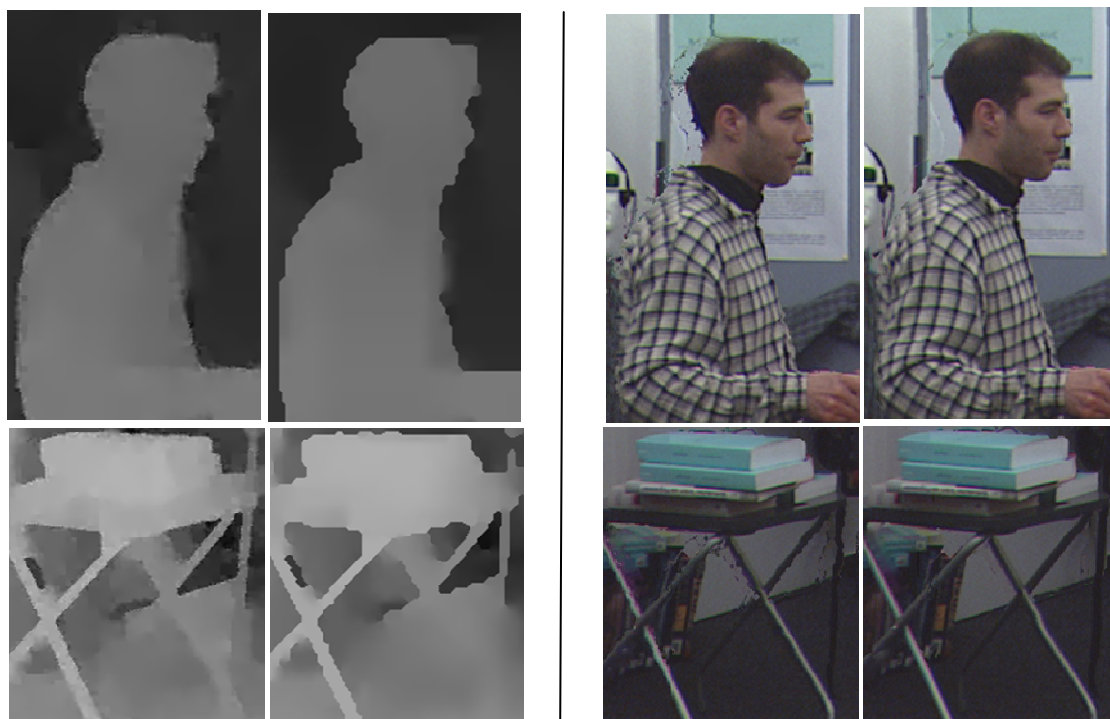
Decoded depth when applying quantization suggested in Pasteau et al. Decoded depth when applying our proposed strategy.
