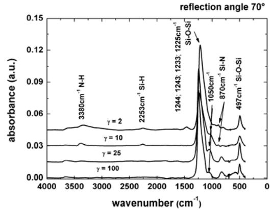
Figure 4. FTIR absorbance spectrum of the singly deposited layers with different  $\gamma$ -values ( $\gamma = 100, 25, 10$  and  $\gamma = 2$ ) recorded in reflection mode at reflection angle of  $70^\circ$ .
