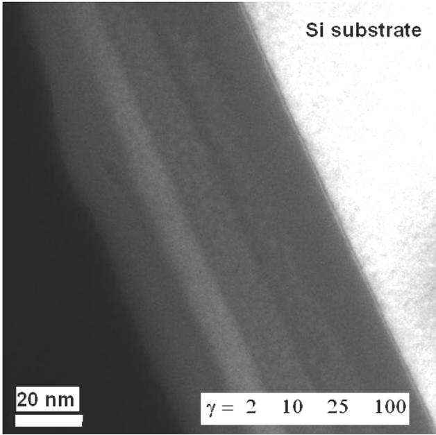
Figure 2. EFTEM image of the multi-layer structure.
