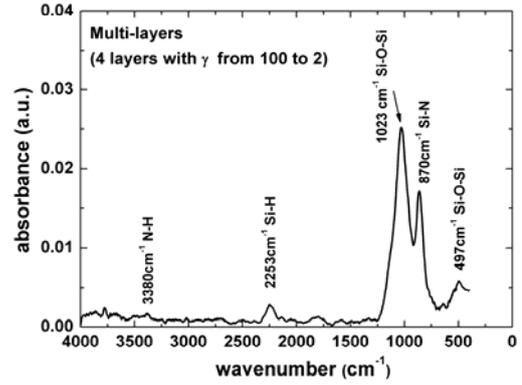
Figure 3. FTIR absorbance spectrum of the multi-layer structure.
