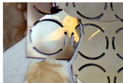
Fig. 5: photography of an example of crack after DRIE
