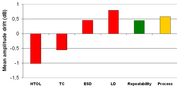
Fig. 15. Emission spectrum mean amplitude drifts after various reliability tests
