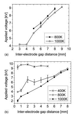
FIG. 9. (a) Measured C-G transition voltage as a function of d for different  $T_0$ , and (b) measured voltage for the transition to spark (N-S, C-S, and G-S) as a function of d for different  $T_0$ . f=30 kHz, and v=1.6 m/s.
