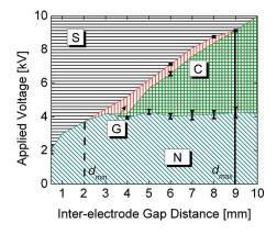
FIG. 8. (Color online) Discharge regime map according to applied voltage as a function of gap distance.  $T_0$ =1000 K, f=30 kHz, and v=1.6 m/s. S: Spark, G: Glow, C: Corona, and N: No discharge.
