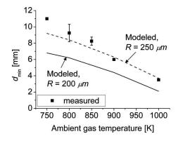
FIG. 17. Comparison between measured and modeled  $d_{\min}$  as a function of the ambient gas temperature. f=30 kHz. The experimental data are taken from Fig. 10(a).
