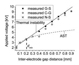
FIG. 16. Comparison of experimental N-S, C-G, and G-S transition voltage and modeled thermal instability threshold and AST, as a function of interelectrode gap distance.  $T_0$ =1000 K and f=30 kHz. The experimental data are taken from Fig. 8.
