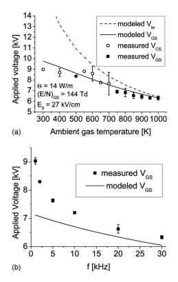
FIG. 14. Comparison of experimental C-S and G-S and modeled G-S transition voltage as a function of (a) ambient gas temperature and (b) pulse repetition frequency. The experimental data shown in (a) are assembled from data shown in Figs. 2, 5, 8, and 9 for the conditions d=5 mm, f=30 kHz, and v=1.6 m/s. The experimental data shown in (b) are taken from Fig. 2;  $T_0=1000 \text{ K}$ , d=5 mm, and v=1.6 m/s.
