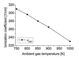
FIG. 11. Calculated ionization coefficient at anode tip for NRP glow discharge at  $d_{\min}$  as a function of the ambient gas temperature, using the measured values of  $d_{\min}$  and of the applied voltage from Fig. 10.
