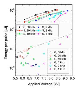
FIG. 4. (Color online) Measured energy per pulse for the glow (hollow) and spark (solid) regimes as a function of applied voltage for f=1-30 kHz.  $T_0=1000$  K, d=5 mm, and v=1.6 m/s.
