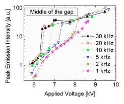
FIG. 3. (Color online) Measured peak emission intensity of N<sub>2</sub> C-B (0,0) in the middle of the discharge gap as a function of  $V_p$  for f=1-30 kHz.  $T_0 = 1000$  K, d=5 mm, and v=1.6 m/s.
