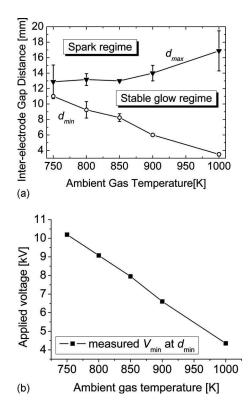
FIG. 10. Measured range of gap distances that permit stable operation of the glow regime (a), as a function of gas temperature and applied voltage at minimum gap distance ( $V_{min}$ ) (b), with f=30 kHz and v=1.8 m/s fixed.
