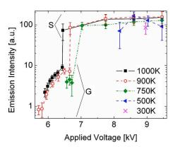
FIG. 6. (Color online) Measured N<sub>2</sub> C-B (0,0) peak emission intensity in the middle of the discharge gap as a function of the applied voltage for  $T_0$  = 300–1000 K. *f*=30 kHz, *d*=5 mm, and *v*=1.6 m/s.
