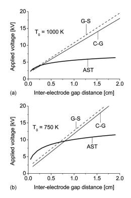
FIG. 15. Theoretical curves at (a)  $T_0$ =1000 K and (b) 750 K for the applied voltages, as a function of interelectrode gap distance for the AST, breakdown for the C-G transition, and the thermal ionization instability for the G-S transition.
