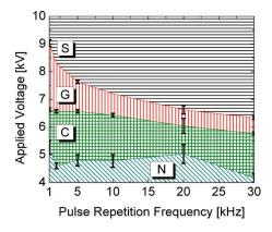
FIG. 2. (Color online) Discharge regime map according to applied voltage  $(V_p)$  as a function of pulse repetition frequency (*f*).  $T_0=1000$  K, *d* = 5 mm, and v=1.6 m/s. S: Spark, G: Glow, C: Corona, and N: No discharge.
