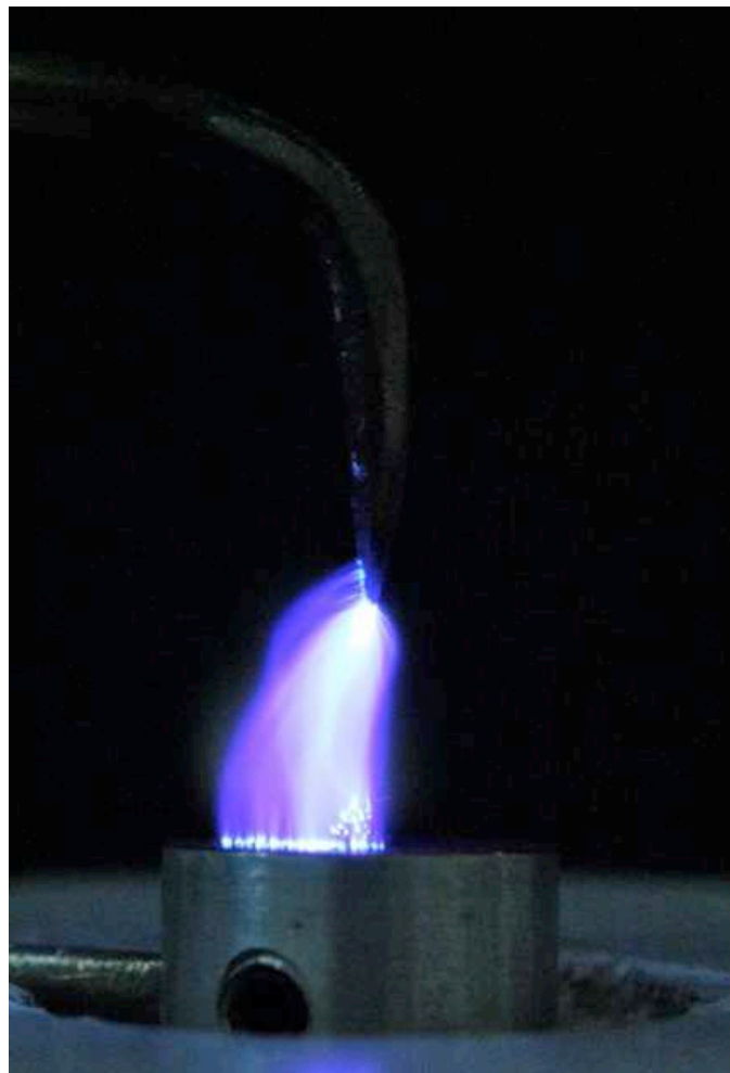
Fig. 1. Nanosecond Repetitively Pulsed plasma discharge (spark), without flame (left) and interacting with a lean flame (right). Characterization of the discharge: f = 30 \text{ kHz} , V = 6.0 \text{ kV} .
