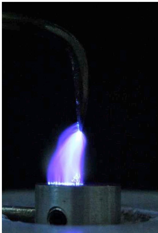
Fig. 1. Nanosecond Repetitively Pulsed plasma discharge (spark), without flame (left) and interacting with a lean flame (right). Characterization of the discharge: f = 30 kHz, V = 6.0 kV.
