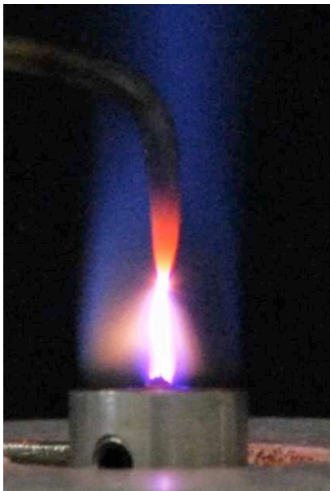
Fig. 1. Nanosecond Repetitively Pulsed plasma discharge (spark), without flame (left) and interacting with a lean flame (right). Characterization of the discharge: f = 30 kHz, V = 6.0 kV.
