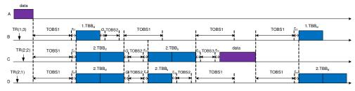
$TR(k_d; k_s)$ : Transmission Request to send a frame which has a dynamic priority  $k_d$  and a static priority  $k_s$ .
