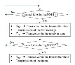
Fig. 3. Principle of the BB-sta protocol.
