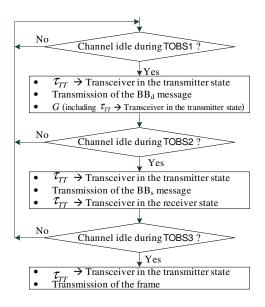
Fig. 6. Principle of the BB-hyb protocol.
