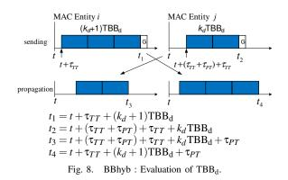
*TOBS2 duration:* Again we consider the type of analysis for TOBS2 in BB-sta (Sect. III-A). Considering Fig. 8, in the loser (MAC entity *j*), the overtaking of the BB<sub>d</sub> message (sent by this loser) by the BB<sub>d</sub> message coming from the winner (MAC entity *i*) is  $(t_4 - t_2)$ . This excess includes G and TOBS2, then we have the value of TOBS2:
