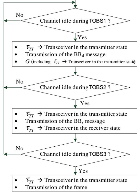
**Figure 5. Principle of the BB-hyb protocol.**
