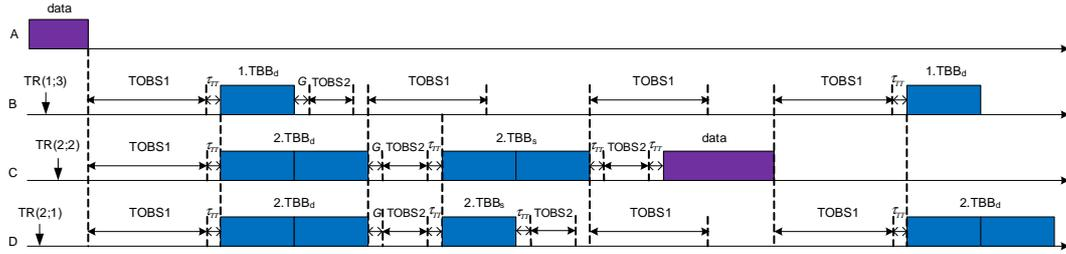
TR( $k;h$ ): Transmission Request to send a frame which has a dynamic priority  $k$  and a static priority  $h$ .
