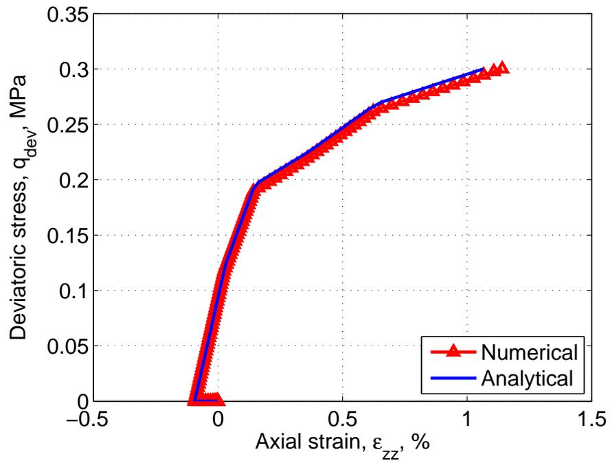
Fig. 2. Variation of the deviatoric stress with respect to the axial strain in case of quasistatic triaxial loading of a cylindrical sample with unit radius and length
