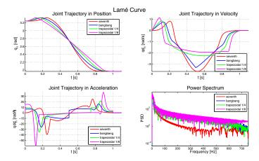
FIGURE 8. Lame curve joint space trajectory and spectral content
