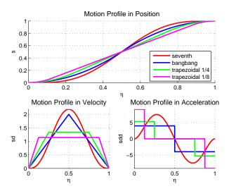
**FIGURE 7**. Motion profiles generated for  $t_f = 1$
