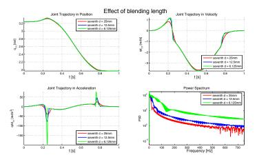
**FIGURE 11**. Spectral content for seventh-lamé trajectories for symmetric blending lengths of d = 25mm, d = 12.5mm and d = 6.125mm
