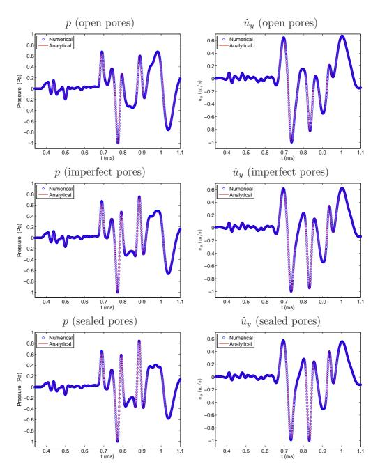
Figure 8: N=4 interfaces, with open pores (top), imperfect pores (middle) and sealed pores (bottom). Time evolution of the acoustic pressure p at recorder R3 (x=1, y=0.02) m (left) and that of the vertical velocity  $\dot{u}_y$  at recorder R4 (x=1, y=-0.112) m (right).
