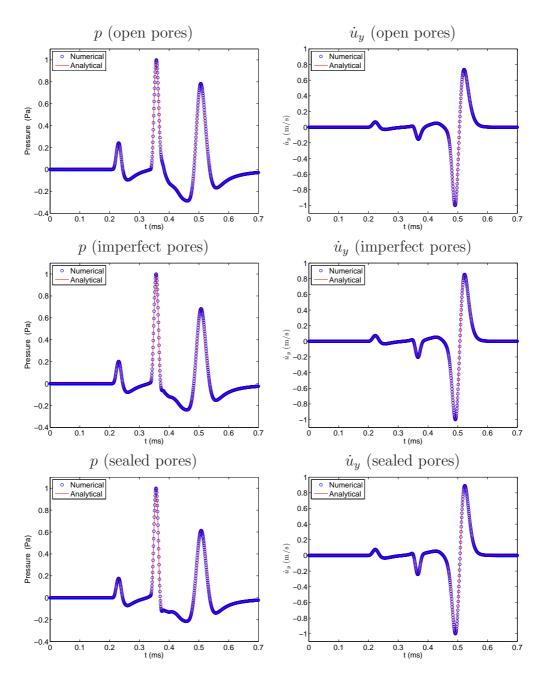
Figure 5: N=1 interface, with open pores (top), imperfect pores (middle) and sealed pores (bottom). Time evolution of the acoustic pressure p at recorder R1 (x=0.5,y=0.02) m (left) and that of the vertical velocity  $\dot{u}_y$  at recorder R2 (x=0.5,y=-0.012) m (right).
