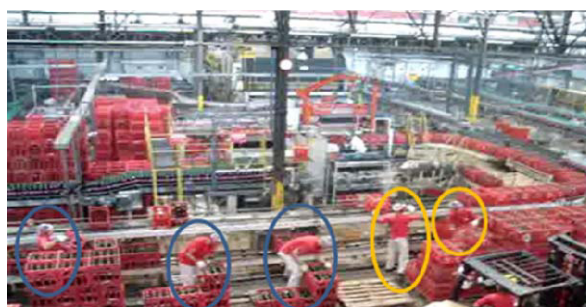
Fig. 4 : Presence of three operators at the loading station instead of two.
