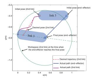
Fig. 4. Task execution of the two tasks: the end-effector,  $x_1$ , and the 2nd link,  $x_2$ , of the 3 DOF planar robot with different priorities. The final position of the 2nd link, which has the lower priority, does not reach its goal position but to the closest position from the desired position in the reachable positions (the circle centered at the final position of the end-effector).
