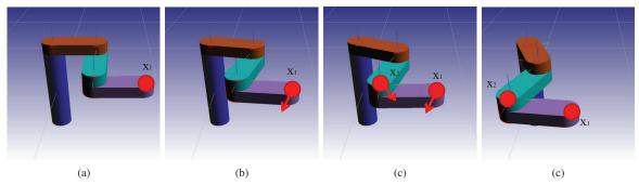
Fig. 1. 3 DOF planar robot simulation: there are two task sets,  $x_1$  and  $x_2$ . (a) initial position of 3-DOF planar robot (b) positioning task of the end effector with high priority,  $x_1$ , is being executed without the other task,  $x_2$ . (c) Positioning task of 2nd link,  $x_2$ , is added with a lower priority. (d)  $x_1$  and  $x_2$  are executed with priorities.
