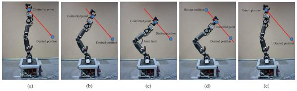
Fig. 7. Joint limit task execution of the 7 DOF manipulator with positioning and orientation tasks. (a) Initial position of 7-DOF manipulator (b) Positioning and orientation tasks,  $x_2$ , execution without joint limit (c)  $x_2$  execution with joint limit (d) Return positioning task,  $x_2$ , execution as elbow joint is extricated from joint limit (e) Final position of 7-DOF manipulator
