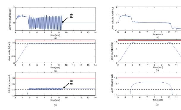
Fig. 8. Oscillation and instability due to the discrete task transition. When the activation border is reached, joint limit task is inserted with a higher priority, the oscillation starts due to the discrete task transition. The experiment is terminated at around 9.4 seconds due to the instability of the robot. (a) Joint velocity. (b) Elbow joint angle near the activation border. (c) Elbow joint angle plotted in a smaller scale (zoom-in view). The joint angle oscillates around activation border.
