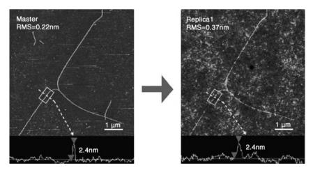
**Figure 1.5** Demonstration of single-wall carbon nanotube reproduction using UV-NIL. (Reproduced with permission from [30]. Copyright © (2004) American Chemical Society.)
