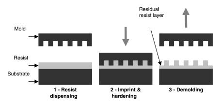
Figure 1.1 Schematic of the nanoimprint process.
