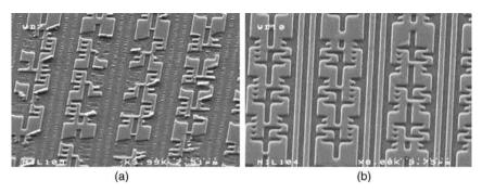
Figure 1.9 Resist imprinted with an untreated (a) and a treated (b) mold under otherwise the same conditions.
