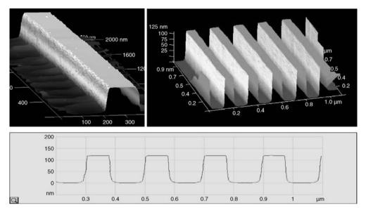
**Figure 1.8** Example of mold characterization by three-dimensional atomic force microscopy (AFM3D) (100 nm wide lines).
