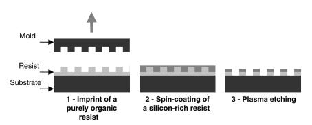
Figure 1.2 Schematic of the S-FIL/R nanoimprint process.
