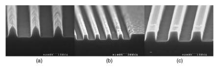
**Figure 1.7** Examples of silicon etched with different UV-NIL resists in exactly the same conditions: (a) purely organic resist; (b) silicon-containing resist; (c) perfluorinated resist.
