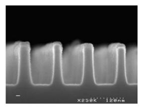
**Figure 1.6** Example of 40 nm wide lines etched 120 nm deep in silicon using a silicon-containing resist, before removing the resist residue.
